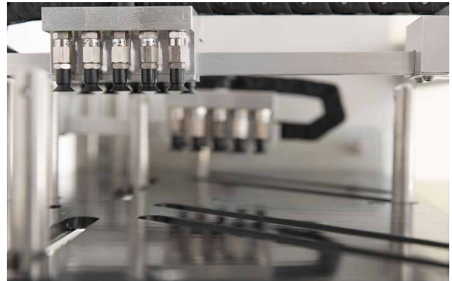
The two heads of the stack loader.
