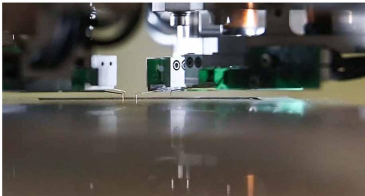
tips about the same amount. One set of probe tips are used on all jobs needing that type of needle until they need replacement. Operating cost can then be predictable for a given production load.
