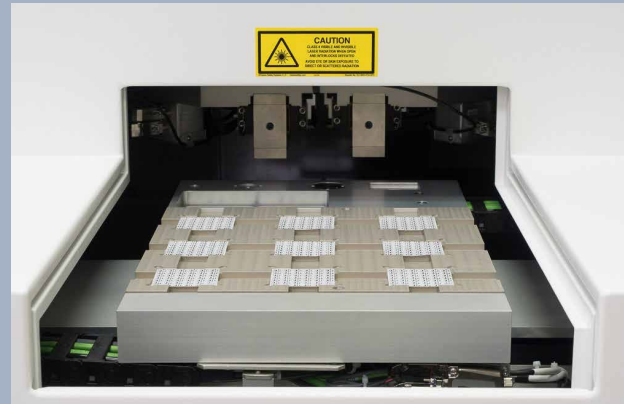
Standard flat vacuum chuck on the left and a custom fixture for a 3x3 array of substrates on the right.
